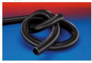
Material: PVC self-supporting profile, open geometry, very light. Temperature: -25 to + 65C extraction hose, crush resistant - for industrial vacuum cleaners and home. Diameter range: 25, 32, 38, 40, 50 mmLength of storage: 30 m.b.Options occurrence:Standard (gray), AS (black anti-static), EC (black electrically conductive).
