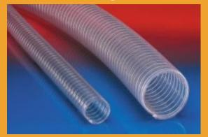
Material: PVC, braided stainless steel wire spring. The wall thickness of 3 to 7 mm in depends on the diameter. Temperature: -20 to + 70C (briefly + 80C) Heavy execution, suction and discharge hose, smooth inside and outside, very good resistance to pressure and vacuum. Diameter range: 10 to 102 mmLength of storage: 30 and 60 m.b. (10-35 mm diameters).
