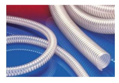
Material: Soft PVC wall, hard PVC braid, The wall thickness of from 4 to 6mm depends on the diameter Temperature: -5 to + 7oC (briefly + 8oCIndustrial hose, smooth insideDiameter range: 32 to 100 mmLength of storage: 25 i 50 m.b. (diameter 10-35mm)
