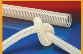
Material: Polyurethane wall, hard PVC braid, The wall thickness of from 4 to 6mm diameter depends on the Temperature: -20 to + 70C (briefly + 80C) Industrial hose, inside smooth, very flexible, hard wearing, anti-static AS-10E9 ohms. Diameter range: 20 to 200 mm Length of storage: 10 and 20 m.b.
