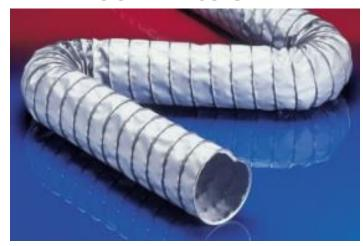
Material and construction: steel strip galvanized clamped on a properly impregnated fabric. Also, multi-layered fabric. Protection against abrasion by external profile. Temperature: -40 to 1100C depending on the material. Temperatures: 170C, 260C, 300C, 400, 600, 900C. Diameter range 38 to 1200 mm depending on the heat resistance. Lengths: Any of 1 m.b.
