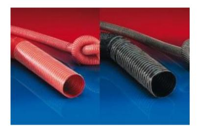
Suction and blast hose to hot and cold air, smooth inside, very flexible, airtight, very light. Length: 4mb SIL - temp. -70 To + 26oC (short-term + 30oC) glass cloth coated with silicone. NEO - temp. -35 To + 135C (short-term + 15oC) glass fabric coated with neoprene.
