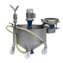
Applied directly to the line, maintains the slurry with constant parameters through the use of a centrifugal pump (internal recirculation mixing by forcing excess pump performance). Practical thanks to wheels allows easy movement, available in 6 different sizes: 500lt, 600lt, 800lt, 900lt, 1000lt, 1200LT
